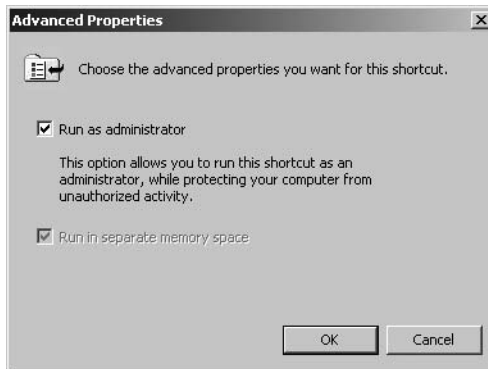
Figure 2-4 To configure the Windows PowerShell shortcut to run with administrative rights, choose the Run As Administrator check box found under Advanced Properties.
