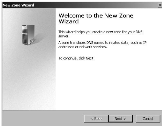
Figure 18-6 New DNS zones are easily created by walking through a seven-page wizard.
